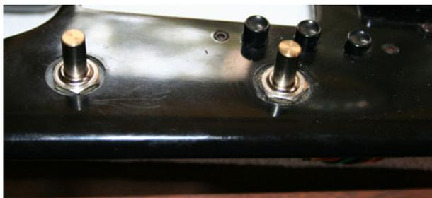
8. Fasten the board using the corresponding washers and nuts.
