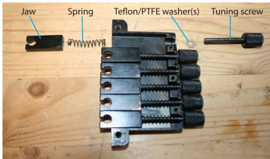
It's not necessary to completely disassemble the trem for lubrication and service on the tuning screws. You can also take them out and reinstall them on the assembled trem. It may be necessary to take off the saddles in this case, to get the jaws out of the tuner housing. However, these pics might give you a better idea of how everything works, and how to remove/reassemble single parts easier.
