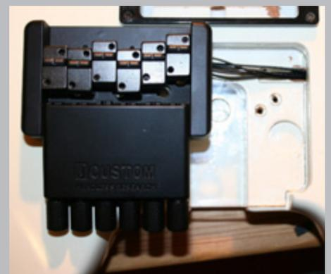
I color-coded the single piezo wires afterwards, using different cable ties. This is not necessary, but helps finding the right wire, if a single piezo doesn't work.
