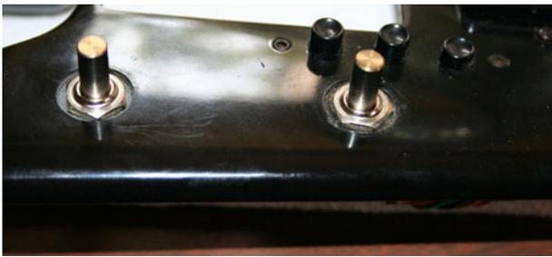
8. Fasten the board using the corresponding washers and nuts.
